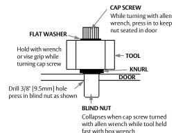
**Diagram 4** End view showing three fastening methods depending on door type.
