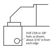
**Diagram 2** Rear view of end piece showing cable routing through end piece.
