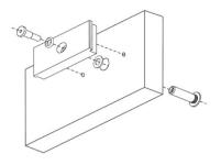
12. LOCATE the armature with roll pins onto the door.
