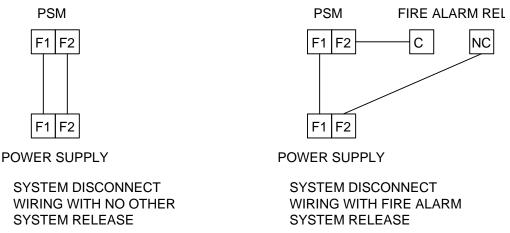
Refer to Figure 2. Terminal F1 in the PSM receives +V power directly from the power supply. Terminal F2 in the PSM connects to F1 in the PSM via an internal 10 Amp relay contact which is closed in the normal condition. So in the normal condition, terminal F2 in the PSM can output +V. In system disconnect, the connection between terminals F1 and F2 in the PSM opens, so there is no voltage on F2.
